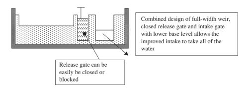
Fig. 4. Improved intake – end view.
