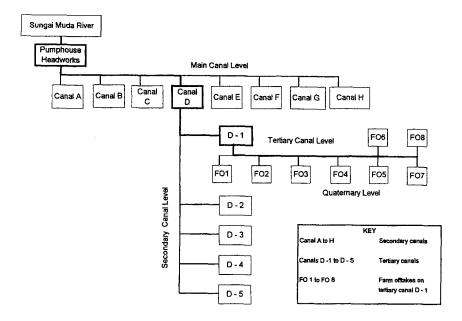
Figure 1. Schematic representation of part of the Sungai Muda Irrigation Scheme showing the path of analysis of design of water control.
