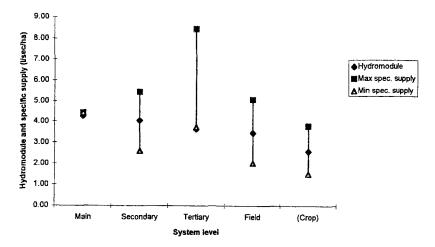
Figure 2. Graph of differences between the required presaturation hydromodule and the actual specific supply (both l/sec/ha) based on gate design approximation of the Sg. Muda Irrigation System.
